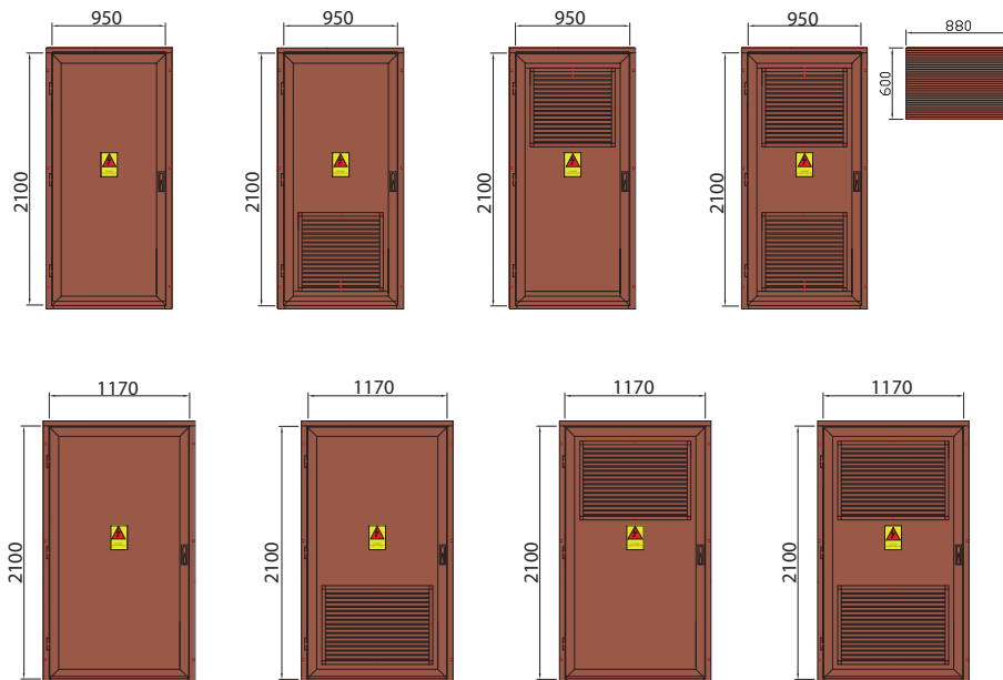
Applications in KSW296/.. Transformer Stations with the height of h- 2970 mm
